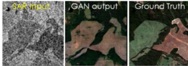
**Figure 2:** Preliminary results show promise toward converting single-band synthetic aperture radar (SAR) images into richer multiband/multicolor images (GAN output).
